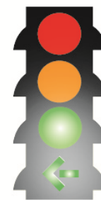
Protected-permissive left-turn signal (Credit: Michele Weisbart)
