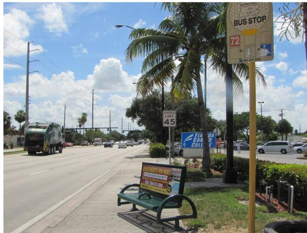
Lack of buffer between sidewalk and street and bench blocking portion of the sidewalk.
