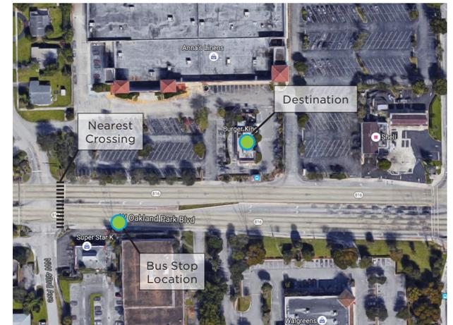
This bus stop is located closer to the destination than the nearest crossing. Many pedestrians were observed crossing mid-block to access the Burger King. Relocating it to the other side of the crosswalk could help to encourage pedestrians to use the crosswalk.
