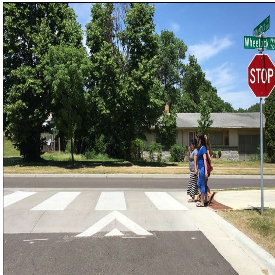
Raised Crosswalks / Speed Tables (Intersection)
