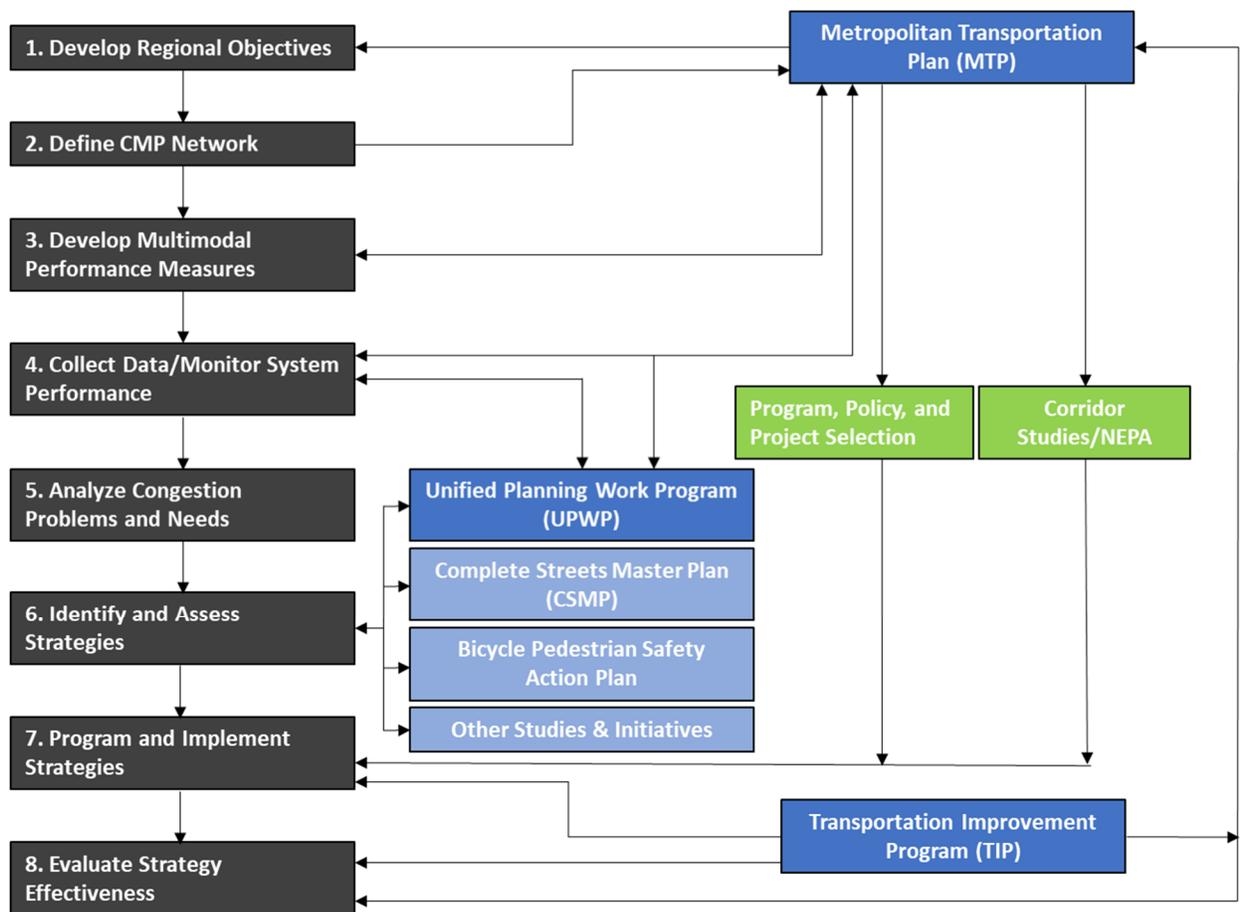
To complement **Figure 4-1**, **Figure 4-2** identifies how the CMP is integrated into various planning functions. With the identification and mitigation of current and future traffic congestion as the foundation of planning and programming decision making, strategies for congestion mitigation are developed on the system level (in the MTP), on the corridor
