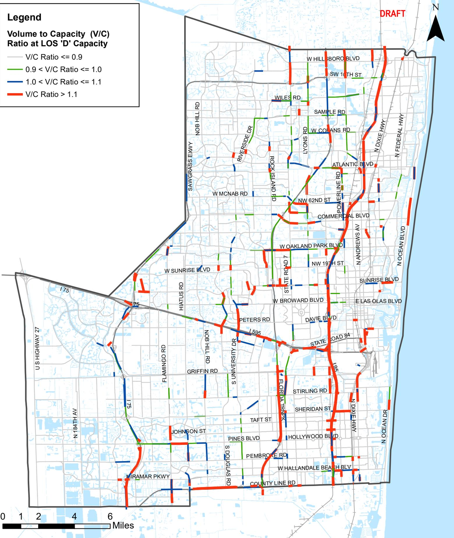
Volume to Capacity (V/C) Ratio at LOS 'D'
