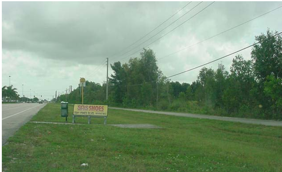
Exhibit 28. At this bus stop, there is no access path from the sidewalk to the road
