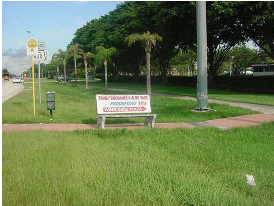
Exhibit 29. The bench is blocking access between the bus stop and the sidewalk
