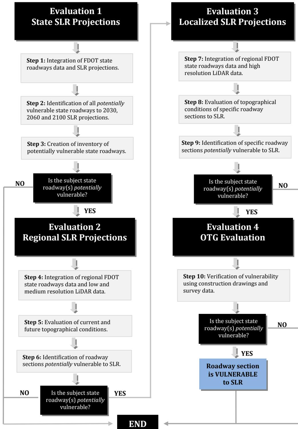
Figure 1: Flow chart of the downscaling evaluation approach developed for the identification of vulnerable state road sections.
