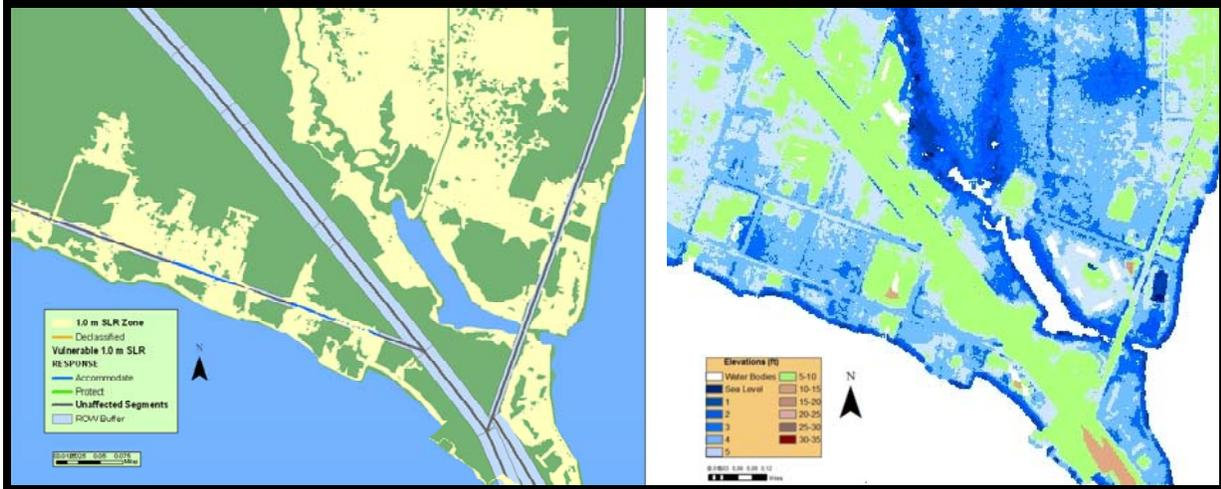
**Figure 26: Comparison of Chapin’s map (to the left) and LiDAR map created in this research (to the right) on the north side of Charlotte Harbor. According to the FAU LiDAR map, this road is not classified as potentially vulnerable. The result is unclear in Chapin’s map.**
