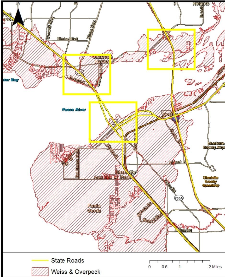
**Figure 24: Weiss and Overpeck crosshatch of Punta Gorda. Red area indicates area with elevations of less than 1-meter, and yellow lines represent state roads. As depicted on the map most of the city is potentially vulnerable.**
