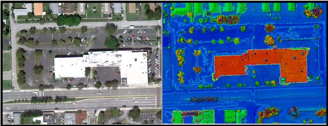
**Figure 17: Building in aerial and LiDAR mapping. The blue areas are below 5 ft NGVD. The mapping shows other features like trees, curbing, and islands in the road.**
