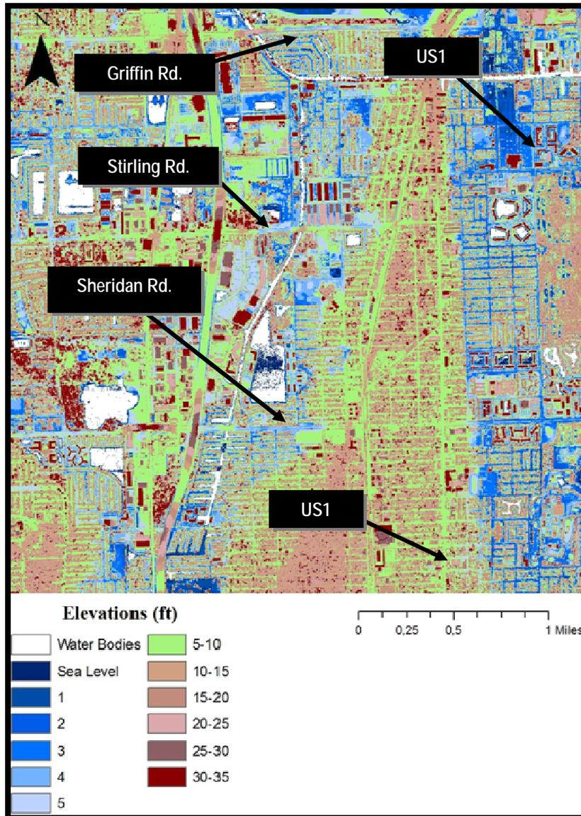
**Figure 16: Dania Beach overlay map using high resolution LiDAR data (7-inch vertical accuracy).**
