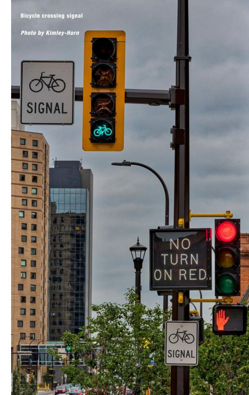
Installation of Bicycle Signals is particularly appropriate at conflict zones or where a bicyclist would otherwise not have a signal facing them, as well as in Contra-Flow and Two-Way Separated Bicycle Lanes.
