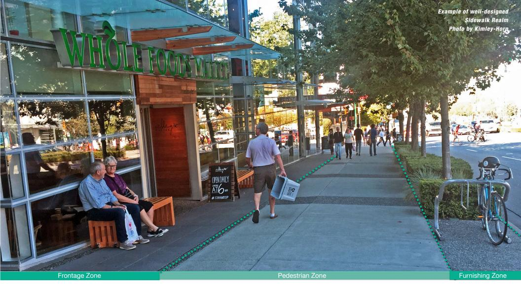
The Sidewalk Realm is located between the curb and the property line. Sidewalks are designed primarily to allow safe pedestrian movement separated from moving traffic. This chapter explores three main zone of the Sidewalk Realm: Frontage Zone, Pedestrian Zone, and Furnishing Zone. In addition, design guidelines are analyzed for the following elements:
