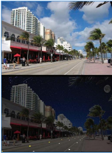
Figure 3 Internally Illuminated Reflective Pavement Marking (IIRPM) Application
