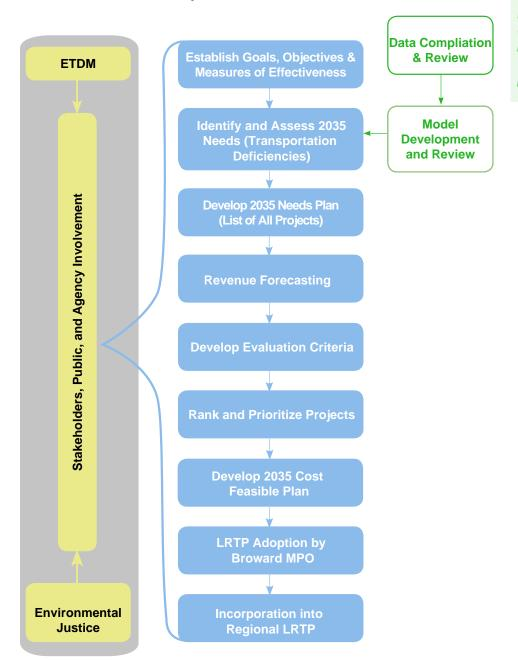
The project selection process used to develop the 2035 Cost Feasible Plan considered intermodal synergies. Exhibit 7 describes the steps in this process.
