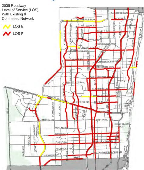
Roadway Level of Service is graded on a scale from A to F.
