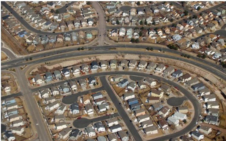
Figure 6-4: Suburban street network has little potential for connectivity (Image source: Alastair Somerville)
