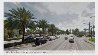
The corridor has a three lanes in each direction. It has intermittent right- and left-turn lanes. It also has a heavily landscaped median and both pedestrian and vehicular lighting. The corridor has 5' - 7' sidewalks and 4' - 5' marked bike lanes. The posted speed is 35 MPH. The land uses mainly consist of new and/or well kept auto-oriented shopping centers set behind large surface parking lots.
