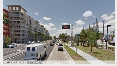
The corridor has a three lanes in each direction. It has intermittent right- and left-turn lanes. It also has median with intermittent landscaping, cobra style vehicular lighting, and dynamic message signs. The corridor has 5' - 7' sidewalks and no marked bike lanes or paved shoulders. The posted speed is 35 MPH. The land uses are redeveloping; new buildings front the street while older buildings and shopping centers are set behind large surface parking lots.
