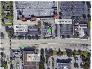
This bus stop is located closer to the destination than the nearest crossing. Many pedestrians were observed crossing mid-block to access the Burger King. Relocating it to the other side of the crosswalk could help to encourage pedestrians to use the crosswalk.
