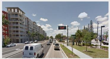
The corridor has a three lanes in each direction. It has intermittent right- and left-turn lanes. It also has median with intermittent landscaping, cobra style vehicular lighting, and dynamic message signs. The corridor has 5' - 7' sidewalks and no marked bike lanes. The posted speed is 35 MPH. The land uses are redeveloping; new buildings front the street while older buildings and shopping centers are set behind large surface parking lots.
