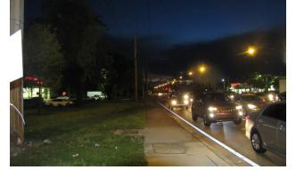
Lighting is poor outside of signalized intersections and present only on one side of the street.
